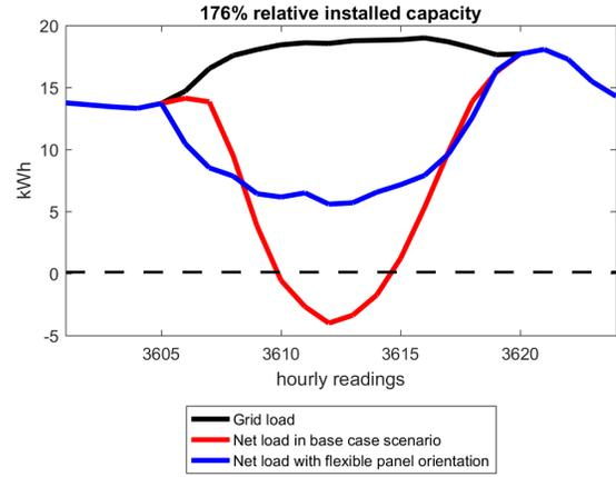
**Figure 1: Flattening the duck curve: the original curve is in red. With optimal choice of orientation, the blue curve shows a substantial reduction in ramping.**
