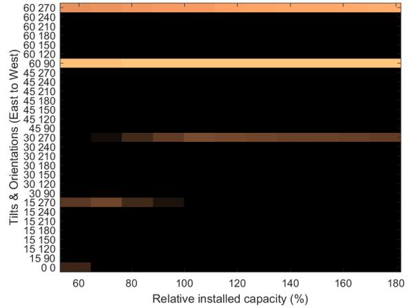
**Figure 2: Optimal orientation. The X axis shows relative installed PV capacity and 0 degree orientation corresponds to North.**
