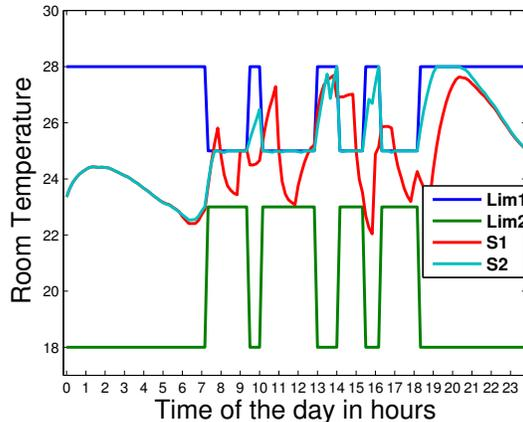
**Figure 1: Room temperature for S1 and S2. Lim 1 and Lim 2 refer to the desirable comfort range based on occupancy.**
