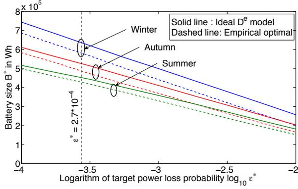
Fig. 4: Accuracy of loss of power formulation: Empirical optimal and Ideal  $D^e$  model battery sizes as a function of target violation probability in three seasons
