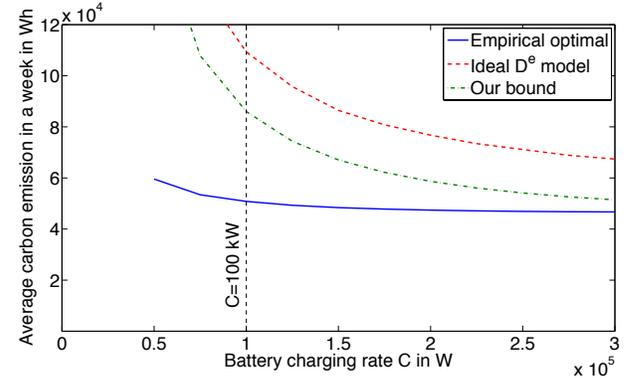
Fig. 7: The impact of charging rate on carbon emission: Carbon emission from genset as a function of battery charging rate  $C$ , and constant battery size  $B = 3 * 10^5 Wh$
