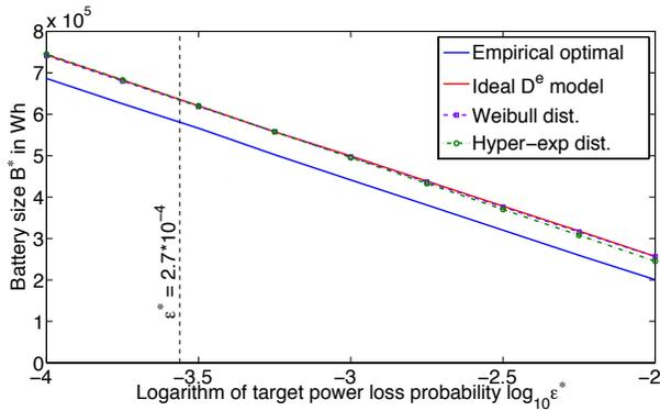
Fig. 5: Accuracy of  $D^e$  modeling: Minimum battery size  $B^*$  as a function of violation probability  $\epsilon^*$ .
