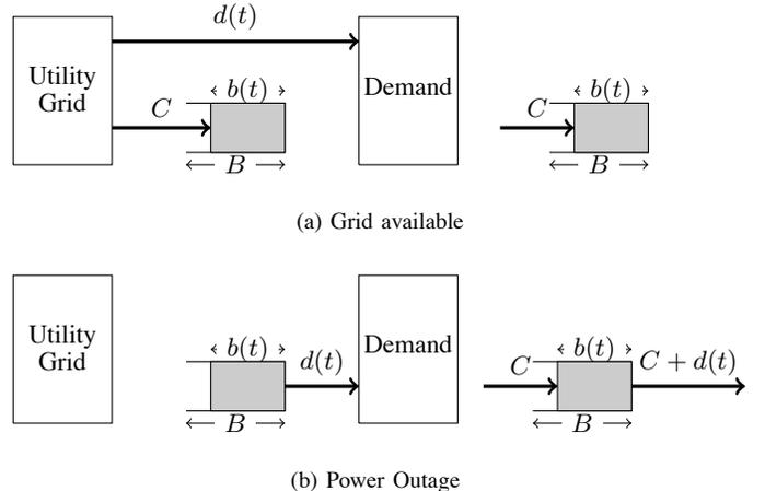
Fig. 3: Storage battery model before and after transformation
