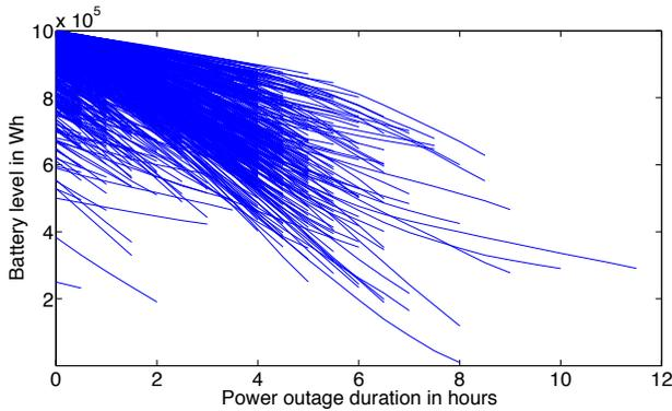
Fig. 1: Trajectories of battery level during load shedding periods for  $B = 1MWh$  and  $C = 10^5W$ .
